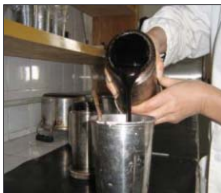
The photos show the flowability of the drilling mud mixture that includes the additive CVR and crude oil. The top photo is without hot rolling and the bottom photo is after hot rolling and cooling (Fig 6).
